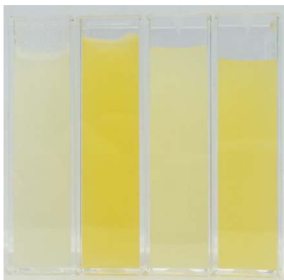
Figure 7: Photographs of whey samples (cuvettes from left to right: uncolored whey, norbixin-colored whey, norbixin-colored whey treated with hydrogen peroxide in the presence of textile-fixed POD, norbixin-colored whey treated with hydrogen peroxide without immobilized POD).
