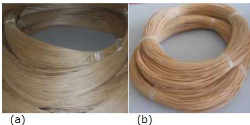
Figure 1: Pictures of tomato yarn—round shape (a) PLA/Ecoflex 50/50 and 15 wt% wood fiber and (b) PLA/Ecoflex 20/80 and 20 wt% wood fiber
