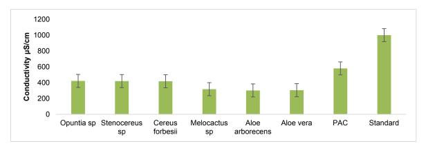
Figure 4: Change on Conductivity using the different samples
