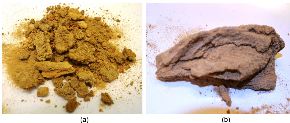
Figure 2: (a) general view of deposit sample #2; (b) close view of some coarse lumps with curved shape and layered structure.
