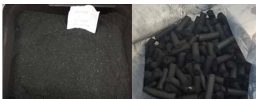
Figure 3: Milled char to be pelletized (left) pelletized biochar (right)
