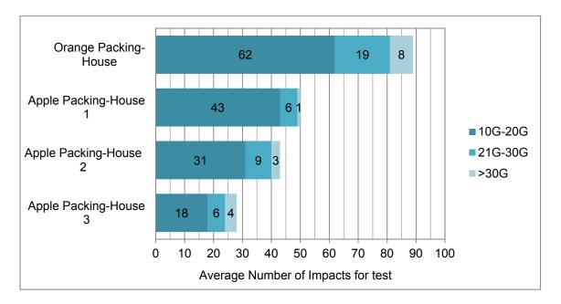
Figure 1: Average number of impacts for three acceleration magnitude ranges measured (10-20G, 21-30 G and >30G) with the Wireless Instrumented Sphere (WIS) in apple (3) and orange (1) packing-lines thru regular fruit flow
