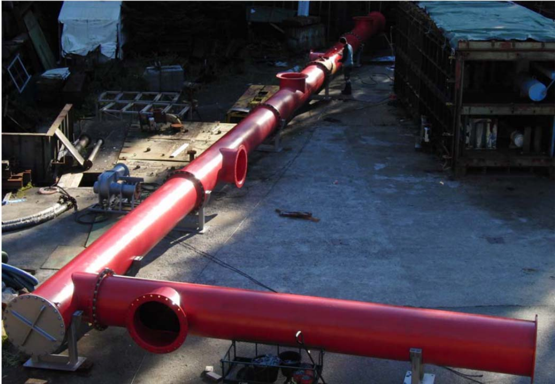
Figure 1: Experimental set-up used for investigating the course of explosions in pipes provided with vents and bends representing exhaust pipes. The diameter of the pipe is 700 mm, the maximum length 36 m.
