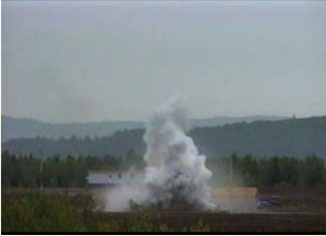
Figure 1: Image of a BLEVE with condensation cloud present (Birk, 2012).
