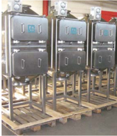
Figure 1: Filter units equipped with cassette filter elements
