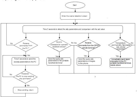
Figure 2: Program flow of the plant safety inspection node device
