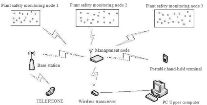
Figure 1: the overall structure of the safety monitoring and alarm system in petrochemical plant
