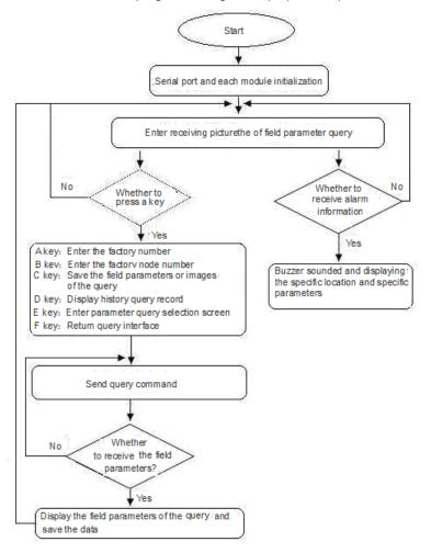
Figure 3: Program flow chart of portable handheld terminal
