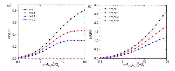
Figure 3: Optimal NSEPs in (a) a single-stage PRO and (b) a multi-stage PRO as a function of  $\gamma$  and r. The log scale is used in x-axis in the plots
