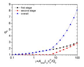
Figure 5: Optimal  $q_d$  at each stage and overall  $q_d$  for the multi-stage PRO process at  $r_1 = r_2 = 0.1$ . The log scale is used in x-axis in the plots
