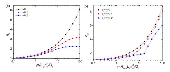
Figure 4: Optimal  $q_d$  in (a) a single-stage PRO and (b) a dual-stage PRO. The log scale is used in x-axis in the plots
