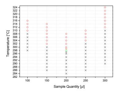
Figure 7: Ignition temperature at different sample volumes for 1-pentanol+water (circle: flammable case; cross: non-flammable case; triangle: the lowest flammable temperature)
