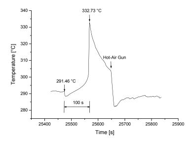
Figure 5: Time history of a typical autoignition experiment (C<sub>5</sub>H<sub>12</sub>O, 200 µl, 292 °C)
