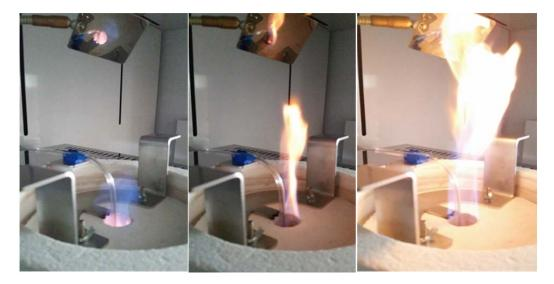
Figure 4: Development of the flames emitted above the top of the flask
