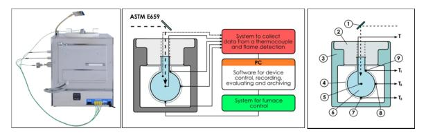
Figure 1: General diagram of the testing system adopted for the AIT tests
