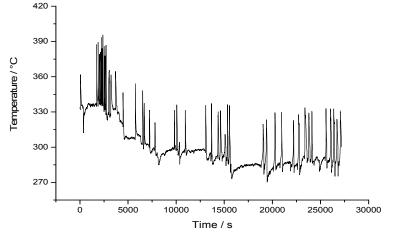
Figure 3: AIT owing to the 1-pentanol recorded at VEC, VSB-TU Ostrava
