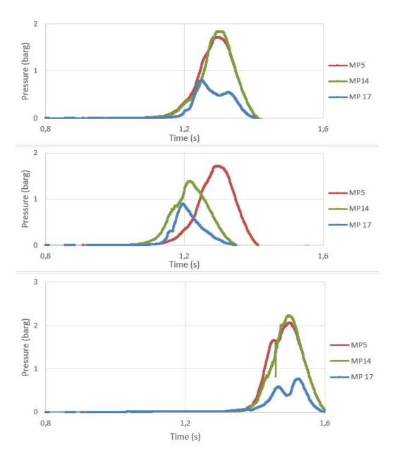
Figure 2: Simulated explosion pressures for different ignition points: mill room(top), classifier(middle) and coal feeder(bottom).
