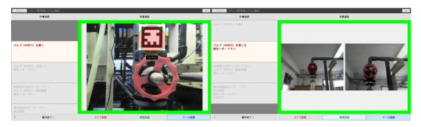
Figure 2. Operation procedures and target device recognition using AR and SURF technology
