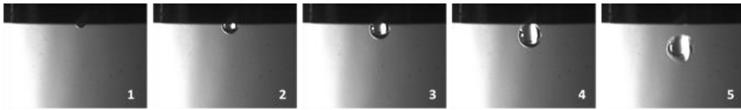
Figure 3: Pictures of droplet formation sequence at 2.4 kV. The elapsed time for pictures 1-4 was 110 ms while picture 5 was taken 10 ms after picture 4
