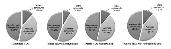
Figure 2: Contents of aromatics, non-aromatics and hetero compounds in tyre-derived oils.
