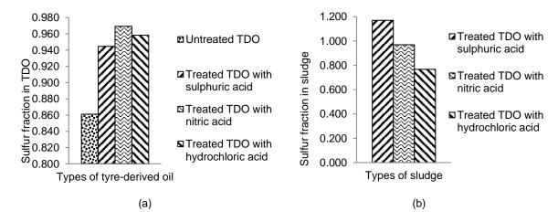
Figure 6: Sulphur content in products: (a) tyre-derived oils (b) sludge
