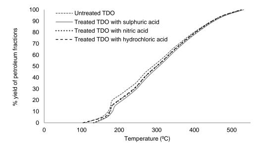
Figure 5: True boiling point curve of untreated and treated tyre-derived oils
