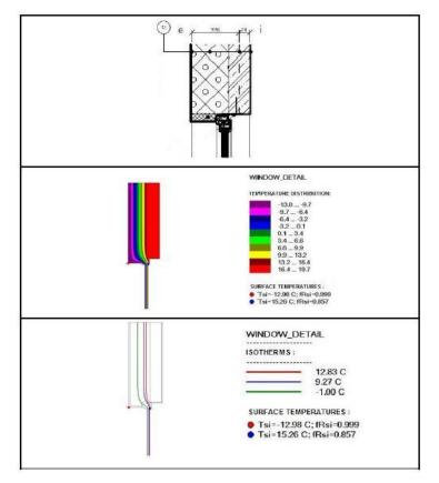
Figure 3: Thermo-physical evaluation of window detail in AREA Software
