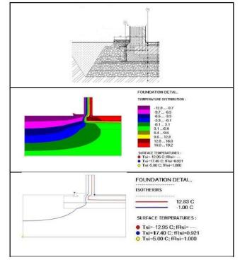
Figure 2: Thermo-physical evaluation of foundation detail in AREA Software
