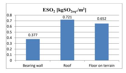
Figure 7: SO<sub>2</sub> emissions of building envelope constructions
