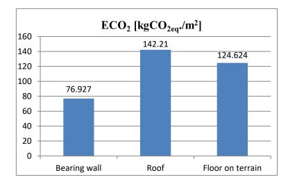
Figure 6: CO<sub>2</sub> emissions of building envelope constructions
