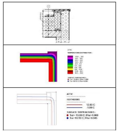
Figure 4: Thermo-physical evaluation of attic detail in AREA Software
