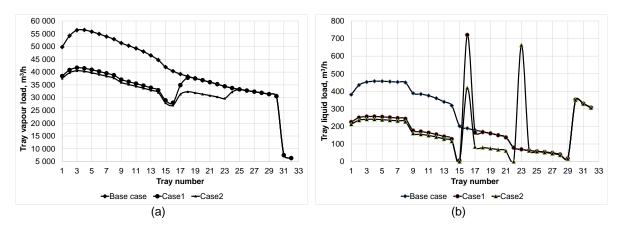
Figure 2: Tray loads of selected cases (a) vapour load, (b) liquid load
