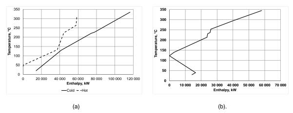
Figure 3: Composite and Grand Composite Curves for Case 1
