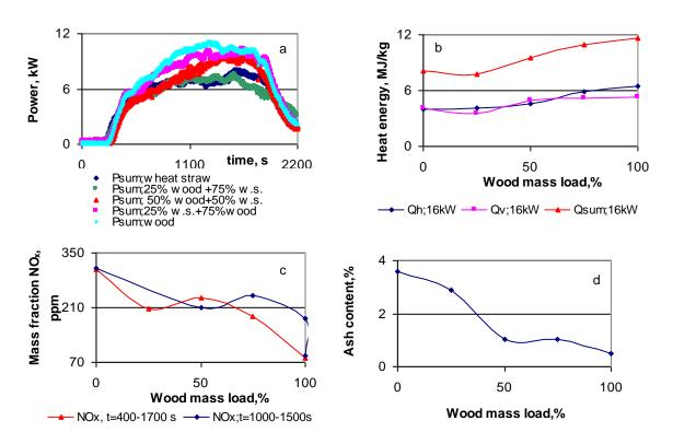
Figure 4: The wood pellets mass load on kinetics of a heat output (a), produced heat energy per mixture mass (b), mass fraction of NO<sub>x</sub> in the products (c) and ash content (d).
