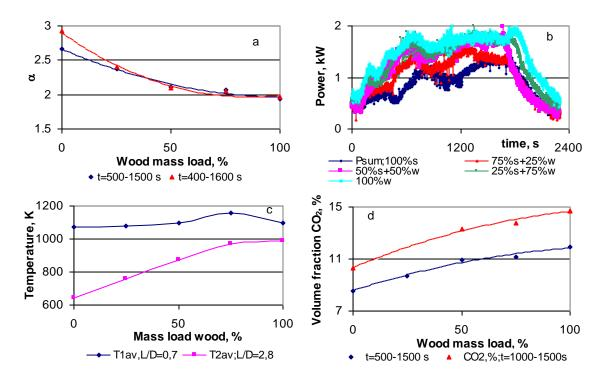
Figure 3: The wood mass load in the mixture with wheat straw pellets on kinetics of the heat output (a) and combustion characteristics (b-d).
