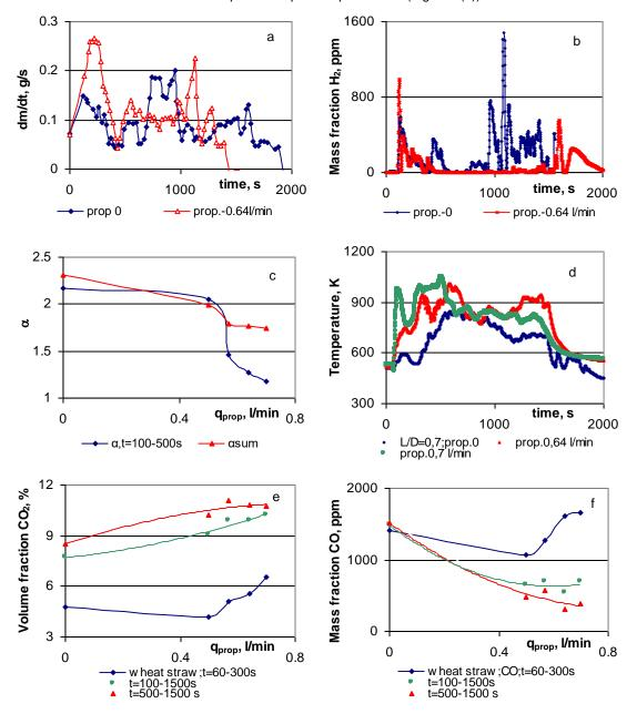
Figure 2: Effect of wheat straw pellets' co-firing with propane on the kinetics of the biomass weight loss rate (a), mass fraction of released  $H_2$  (b), air excess ratio in the reaction zone (c), kinetics of the flame temperature (d) and on the average values of the product composition (e, f).
