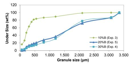
Figure 5: Granule size accumulation at different binder percentage and constant powder ratio of 1/3 (25 % Fine: 75 % Coarse)
