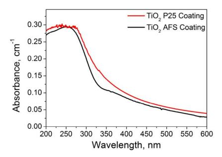
Figure 3: UV-Visible absorption spectra of P25 coating prepared by solvent evaporation technique and AFS  $TiO_2$  coating obtained with a total deposition time of 30 s.
