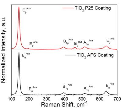
Figure 2: Raman spectra of P25 coating prepared by solvent evaporation technique and AFS TiO<sub>2</sub> coating obtained with a total deposition time of 30 s.
