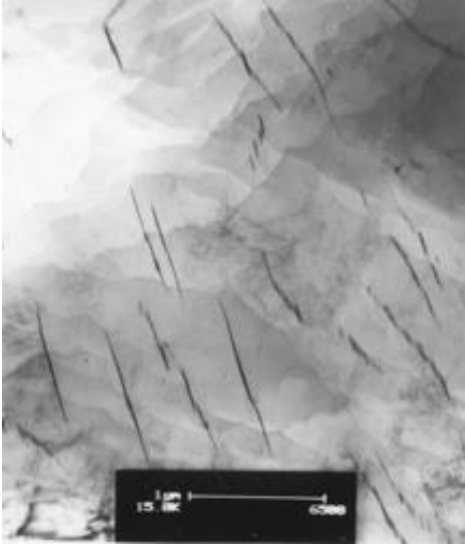
Figure 4: The microstructure in matrix of Mg-4Al-5.1Y-2.5LPC alloy after T6 treatment and after creep (creep temperature 250°C, creep stress 117.1MPa)
