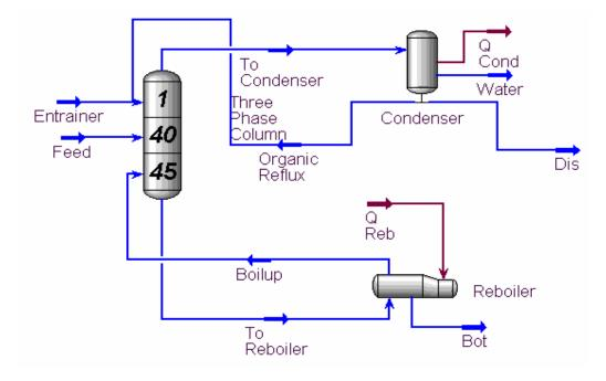
Figure 2: Flow separation method schematic
