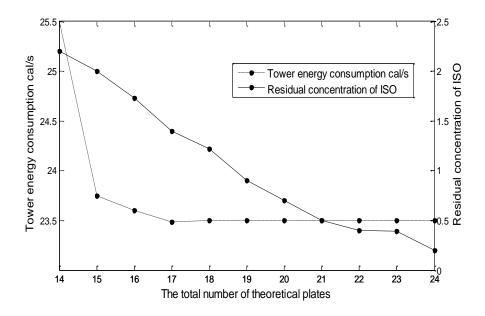
Figure 3: Affect the total number of theoretical plates of the column process indicators
