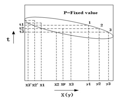
Figure 1: Several partial vaporization and condensation of t-x-y
