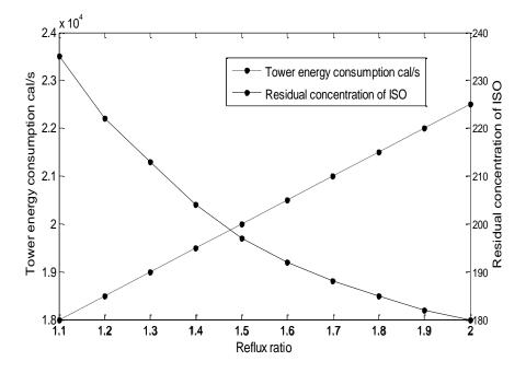
Figure 4: Reflux ratio of column process indicators
