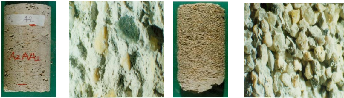
(a) macroscopic features (b) microscopic features Figure 3: Macroscopic and microscopic features of concretion body( W/C 0.8, particle diameter 2~3mm)
