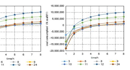
Figure 3: Comparison of coal conservation and emission reduction for different peak load regulation schemes (for 70% capacity of pumped storage units)
