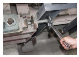
Figure 2: Tensioning Mechanism
