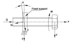
Figure 3: Force Analysis of Bolt
