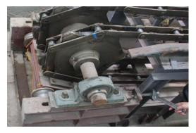
Figure 1: Transmission of Plate-Chain Conveyor
