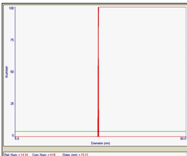
Figure 1: Size distribution of the produced \text{TiO}_2 nanoparticles
