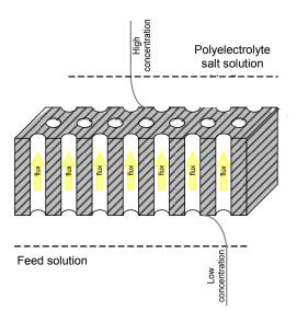
Figure 1: Basic operational principle of a membrane crystallization system: an aqueous solution of polyelectrolyte salt (stripping solution) contacting the hydrophobic membranes is used to generate a partial pressure gradient that drives the transport of solvent from the solution of biomolecules (retentate solution). The progressive removal of solvent induced supersaturation.
