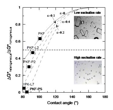
Figure 2: Ratio of Gibbs energy barrier for heterogeneous and homogeneous nucleation as a function of the membrane porosity and the contact angle of lysozyme solution (protein: 40 mg/ml; NaCl as precipitant: 2% w/v). Lines are from equation (2). Abbreviations: PKF - Kynarflex 2800 (polymer); PK- Kynar 460 (polymer); L – LiCl (additive); P- PVP (additive)
