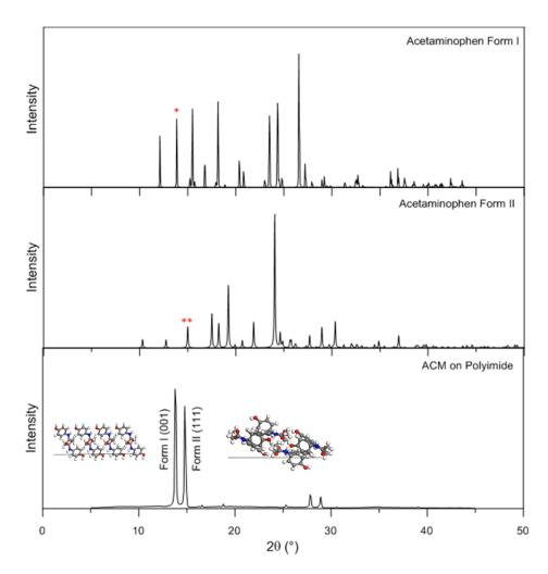
Figure 4: PXRD diffractograms showing concomitant polymorphism in acetaminophen (ACM) crystals grown on polyimide (PI) surface. The experimental pattern is compared to the calculated patterns for ACM Form I (top) and Form II (center) obtained from the crystallographic information files.
