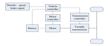
Figure 1: Transmission System Schematic Diagram
