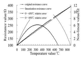
Figure 1: Non-linear errors distribution diagram within the range of 0-650  $^{\circ}$ C and 0-850  $^{\circ}$ C
