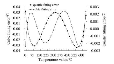
Figure 3: Error distribution of cubic and quartic fitting within the range of 0-650  $^{\circ}C$
