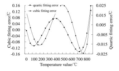
Figure 2: Error distribution of cubic and quartic fitting within the range of 0-850  $^{\circ}C$
