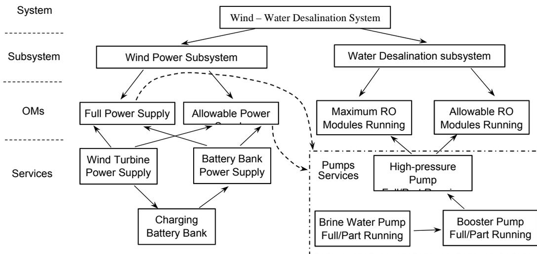
Figure 5: The functional representation of integrated wind-water desalination control system
