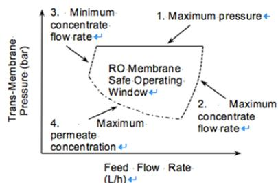
Figure 4: Safe operating window for a RO membrane as proposed by Feron (1985)
