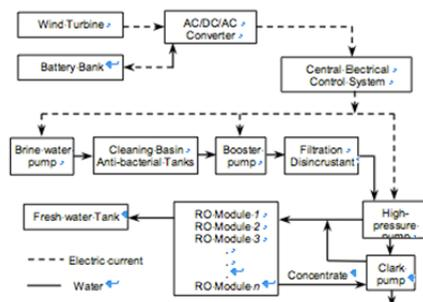
Figure 3: The wind-water desalination system
