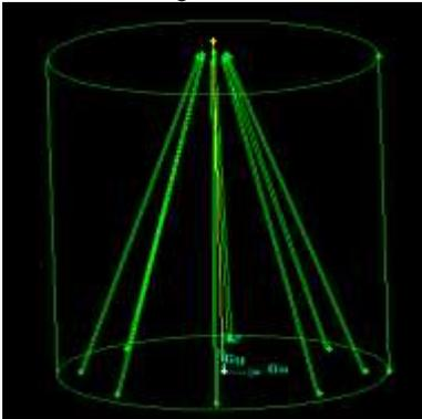
Figure 1: Heat storage model for inclined ground heat exchanger
