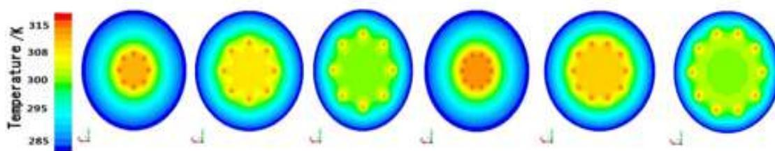
Figure 4: Nephograms of soil temperature field with burial depth of 5m, 10m and 15m using 8 and 10 heat exchangers
