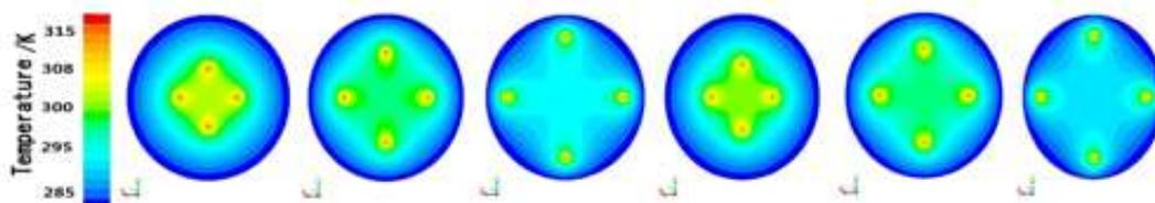
Figure 7: Nephograms of temperature field at different burial depth and 4 different diameter of water-collecting tube
