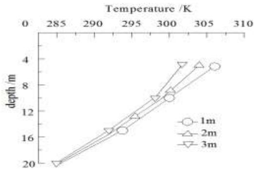
Figure 8: Variation of temperature with depth for different diameter of water-collecting tube after 3 years of continuous heat storage
