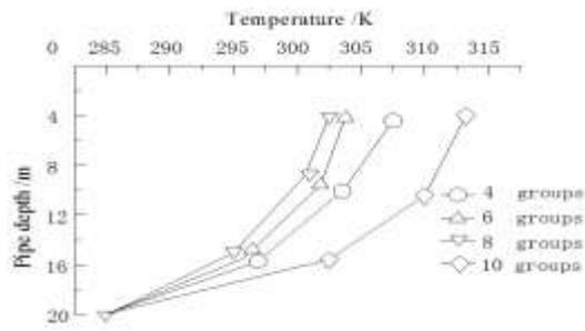
Figure 5: Temperature curve after 3 years of continuous heat storage
