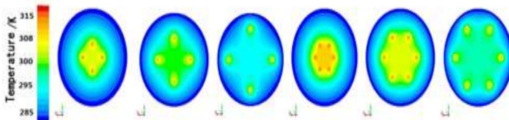
Figure 3: Nephograms of soil temperature field with burial depth of 5m, 10m and 15m using 4 and 6 heat exchangers
