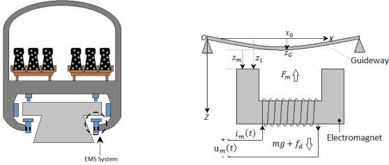
Figure 1: Structure of the MAGLEV train Figure 2: Basic structure of EMS module with flexible guideway
