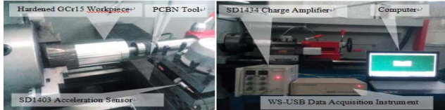
Figure 1 Experimental Cutting Set-up
