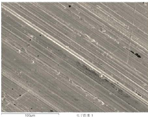
(a) SEM micrograph of MCB sample worn surface
