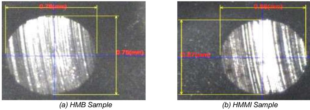
Figure 4: Wear scar diameter of each sample
