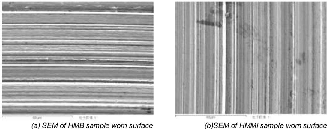
Figure 5: SEM micrographs of worn surface lubricated with different lubricants(upper sample)
