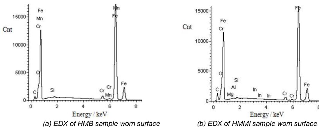
Figure 6: EDX characterizations of the upper sample surfaces
