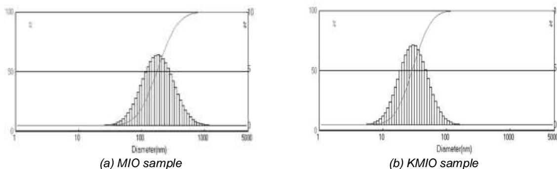
Figure 2: Particle size analysis chart of MIO and KMIO sample
