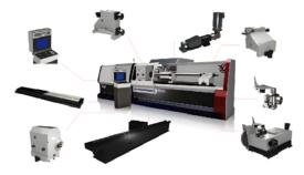
Figure 1: Workpiece moving-CNC roll grinding machine modules
