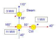
Figure 4: The simple HEN from the Example (after Klemeš et al., 2014)
