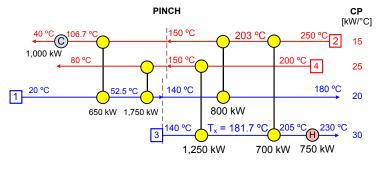
Q<sub>Hmin</sub> = 750 kW Q<sub>Cmin</sub> = 1,000 kW
