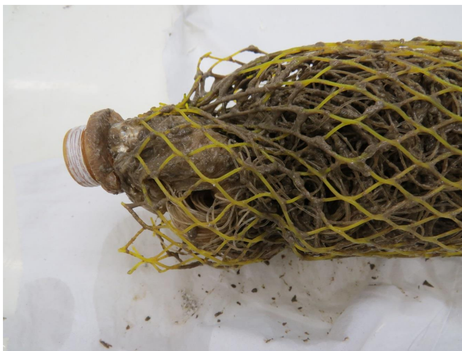
Figure 3: Heat exchange bundle after 5-week experiment with laundry wastewater. There is a great deal of viscous and sticky deposits consisting of biofilm and solid particles on the fiber surface
