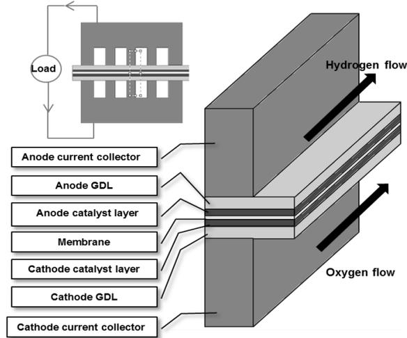
Figure 1: Schematic of the PEM fuel cell
