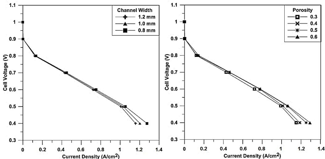
Figure 4: a) Effect of PEM fuel cell channel width, b) Effect of GDL porosity
