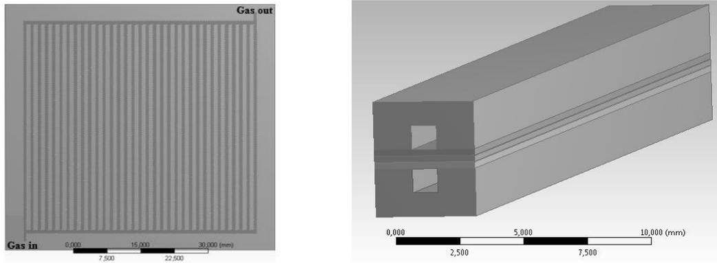
Figure 2: a) Current collector plate with straight channel, b) One straight flow channel of a PEMFC
