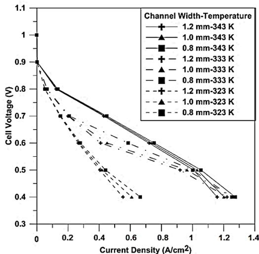
Figure 5: Effect of PEM fuel cell temperature on current density
