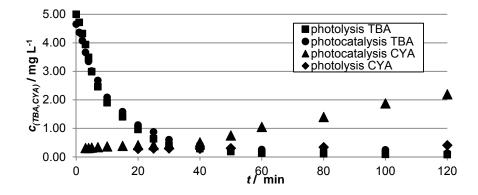
Figure 4. Comparison of photolytic and photocatalytic degradation of terbuthylazine and evolution of the cyanuric acid (Conditions:  $c_{(TBA,0)} = 5 \text{ mg } L^{-1}$ , T = 25 °C, t = 120 min,  $\lambda = 254 \text{ nm}$ , P = 8 W,  $R = 300 \text{ mL min}^{-1}$ , pH = 5)
