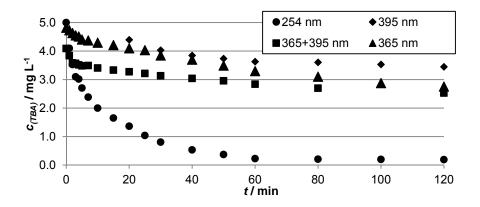
Figure 7. Photocatalytic degradation of terbuthylazine: • 8 W 254 nm, • a 7.2 W 395 nm LED strip placed close to the catalyst, • 8 W 360 nm lamp and 7.2 W 395 nm LED strip placed close to the catalyst  $\blacktriangle$  8 W 360 nm (Conditions:  $c_{(TBA,0)} = 5 \text{ mg L}^{-1}$ , T = 25 °C, t = 120 min, R = 300 mL min<sup>-1</sup>, pH = 5)
