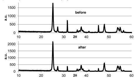
Figure 3. XRD analysis of the TiO<sub>2</sub>/chitosan photocatalyst before and after photocatalytic reaction in the reactor
