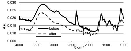
Figure 2. FT-IR analysis of the TiO<sub>2</sub>/chitosan photocatalyst before and after photocatalytic reaction in the reactor
