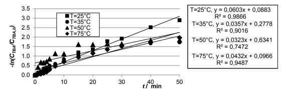
Figure 8. Photocatalytic degradation of terbuthylazine at different temperatures ( $\blacksquare \bullet \blacktriangle \bullet \bullet$  experimental data, line – theoretical data, conditions:  $c_{(TBA,0)}=5 \text{ mg } L^{-1}$ , t = 120 min,  $\lambda = 254 \text{ nm}$ , P = 8 W,  $R=300 \text{ mL min}^{-1}$ , pH = 5)
