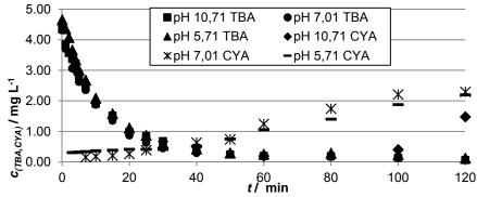
Figure 5. Photocatalytic degradation of terbuthylazine and evolution of cyanuric acid at different pH values (Conditions:  $c_{(TBA,0)} = 5 \text{ mg } L^{-1}$ , T = 25 °C, t = 120 min,  $\lambda = 254 \text{ nm}$ , P = 8 W,  $R = 300 \text{ mL min}^{-1}$ )
