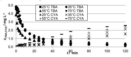
Figure 6. Photocatalytic degradation of terbuthylazine and evolution of cyanuric acid at different temperatures (Conditions:  $c_{(TBA,0)} = 5 \text{ mg } L^{-1}$ , t = 120 min,  $\lambda = 254 \text{ nm}$ , P = 8 W,  $R = 300 \text{ mL min}^{-1}$ , pH = 5)
