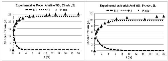
Figure 3. Comparison of trajectories between mechanistic model and experiments.
