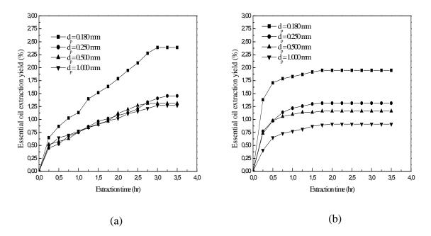
Figure 3: Essential oil extraction yield as a function of extraction time for different particle size, (a) Supercritical CO<sub>2</sub>, (b) Hydrodistillation.
