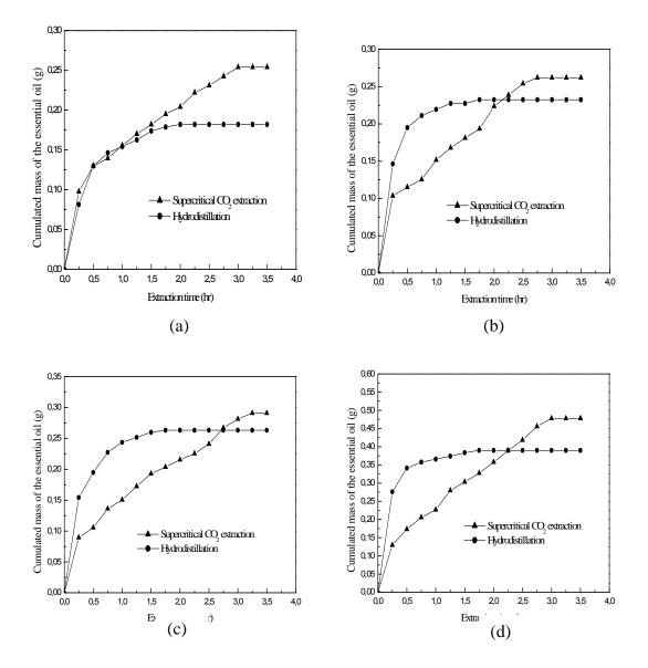
Figure 2: Accumulated mass of essential oil as a function of time obtained by Hydrodistillation and Supercritical CO<sub>2</sub> for different particle size: (a) 1 mm, (b) 0.5 mm, (c) 0.25 mm, (d) 0.18 mm
