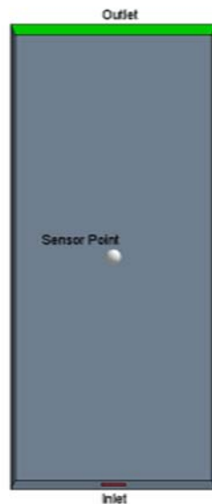
Figure 1: Geometry of the investigated bubble column. The sensor point in the centre ( h = 0.225 m, w = 0.1 m, d = 0.025 m) is used to determine the oscillation frequency and amplitude.
