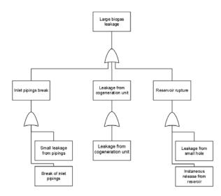
Figure 2: Fault tree for biogas leakage event
