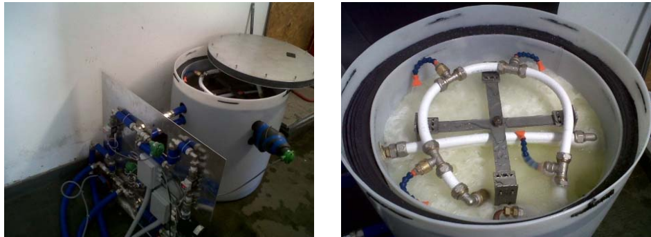
Figure 2 – 5 kWh cold prototype for cold storage by means of PCM
