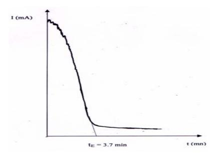
Fig.3. Curve of accelerated scaling for the water of Hamma.
