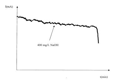
Fig.6. Curve of accelerated scaling for the water of Hamma added with 400 mg/L of soda.
