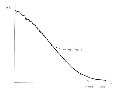
Fig.4. Curve of accelerated scaling for the water of Hamma added with 400 mg/L of Na<sub>2</sub>CO<sub>3</sub>.
