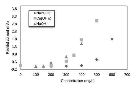
Fig.8. Evolution of the residual current according to the concentration
