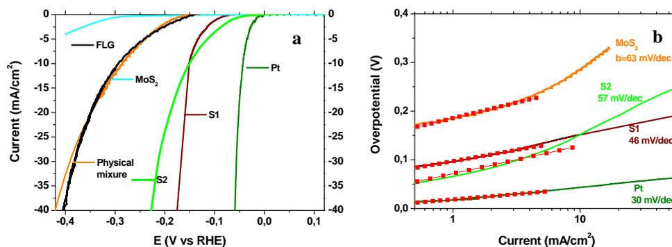
Figure 4. Polarization curves obtained with several catalysts deposited on glassy carbon electrodes (a), and corresponding Tafel plot (b).
