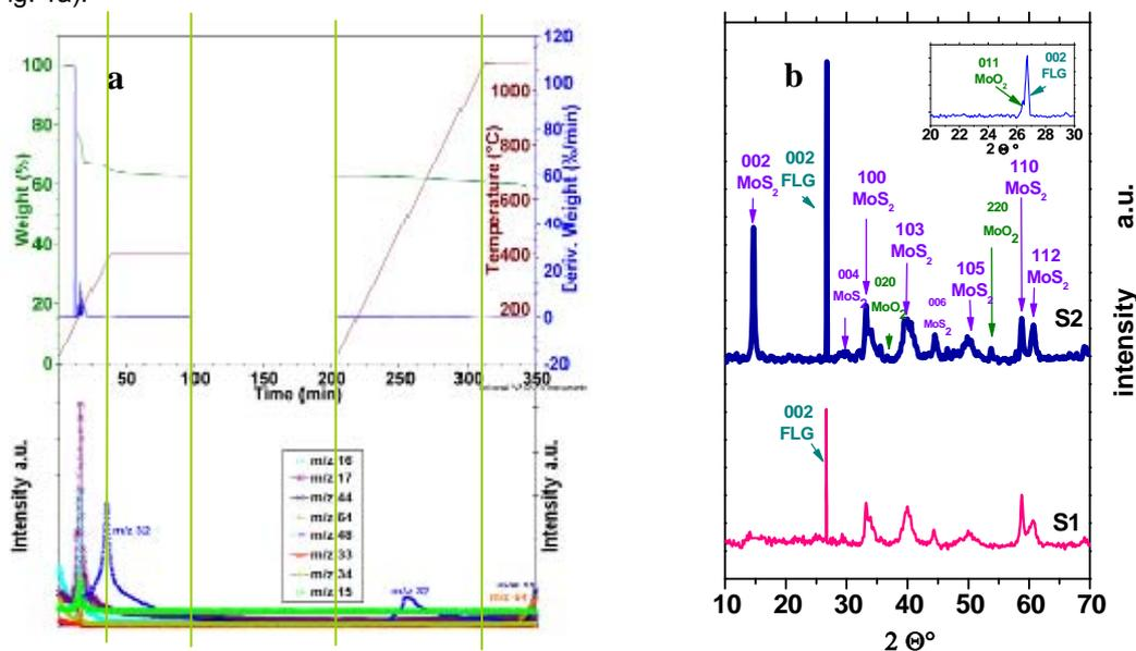
Figure 1. TG-DTG profiles, during the test simulating the S1 synthesis conditions, and the corresponding TIC (a). XRD diffraction patterns of the samples after the two steps of synthesis and for different annealing time at  $1100^\circ\text{C}$  (b).
