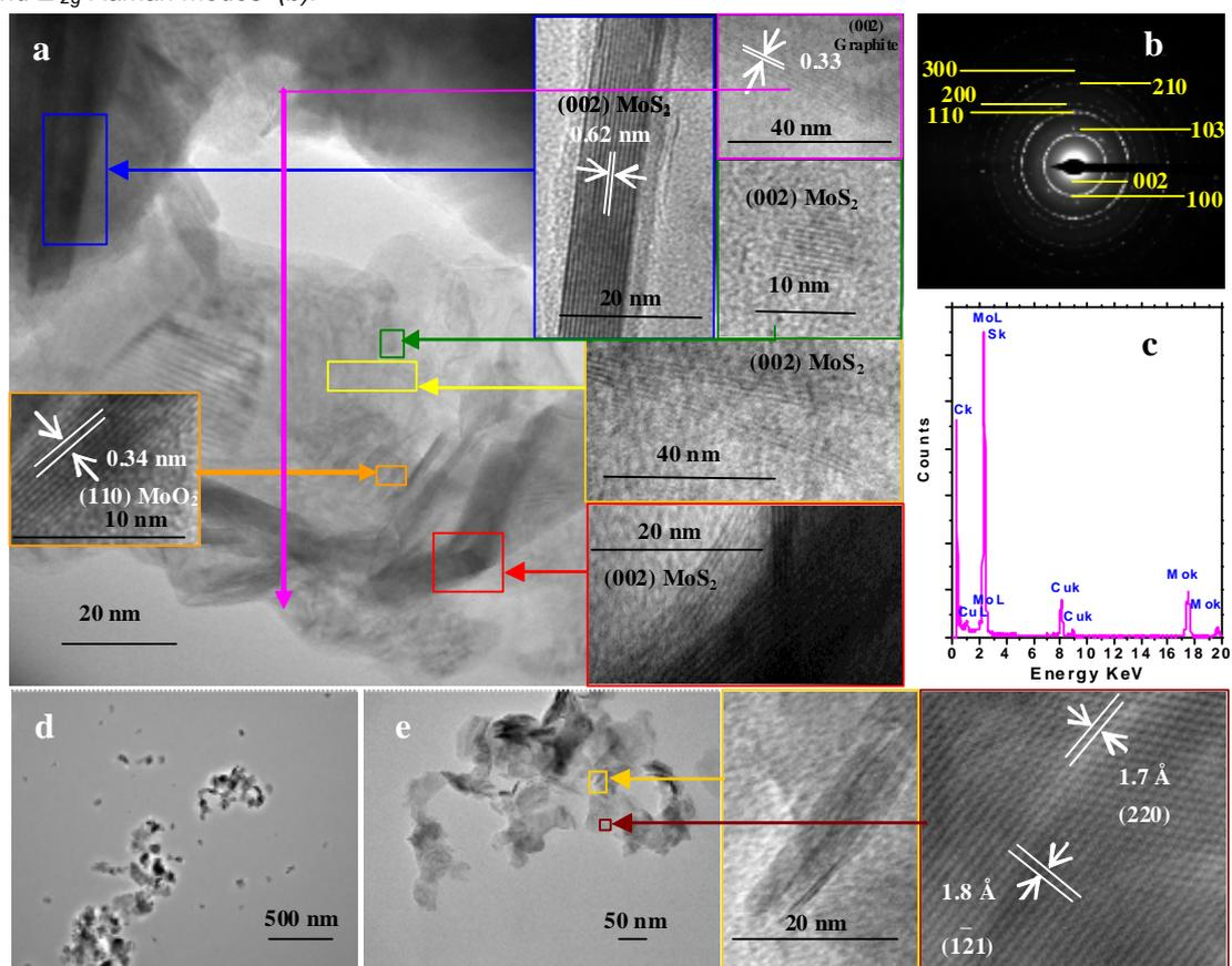
Figure 3. **S2** TEM image (a), high resolution TEM images in the inserts. **S1** SAED pattern (b) and EDS spectrum (c).  $\text{MoS}_2/\text{MoO}_2$  TEM images at different magnification (d,e), high resolution TEM images in the inserts.
