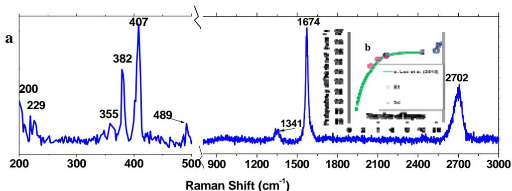
Figure 2. Raman Spectra of **S2** in the range 200-3000  $\text{cm}^{-1}$  (a) and the frequency difference between  $A_{1g}$  and  $E'_{2g}$  Raman modes (b).
