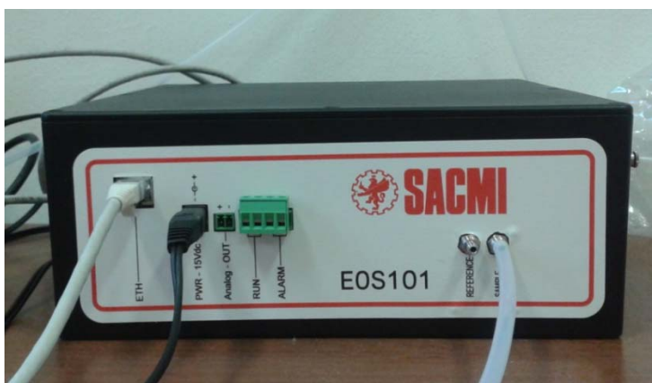
Figure 1 The EOS 101 Electronic Nose
