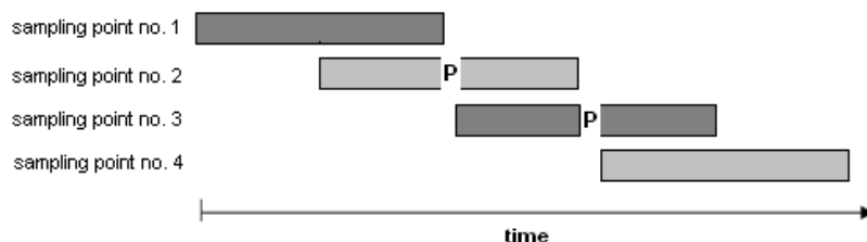
Figure 3: Sampling sequence of odour removal efficiency of the 3-stage treatment unit
